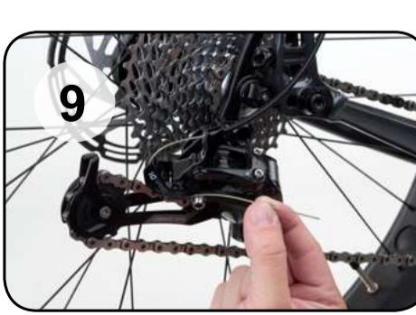
**EN** Feed cable through the shift lever and housing.
