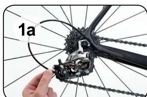
**EN** Measure the length of housing needed. Ensure housing makes smooth arcs and that it seats in the housing stops at a straight angle. The handlebars should rotate completely in both directions without pulling the housing taught.
