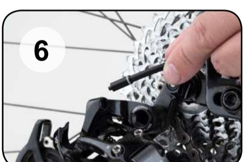
**EN** If there are cable stops on the frame, install lined end caps (B) at those ends of cut housing.
