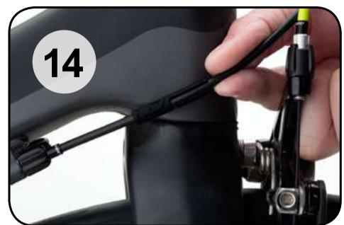
**EN** Install tube tops (E) where the housing rubs against the frame to protect the frame's paint and finish.
