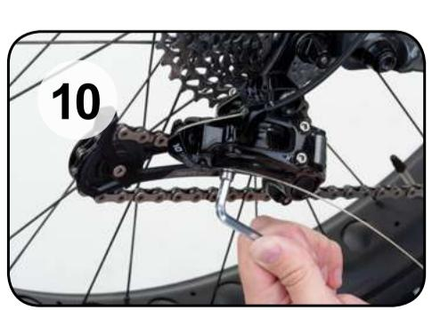
**EN** Tighten anchor bolt and adjust the derailleur per the manufacturer's instructions.
