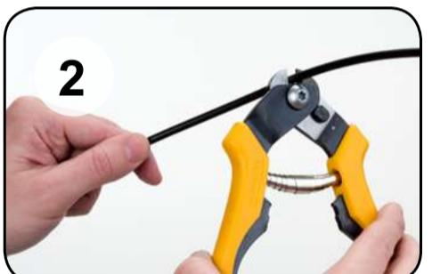
**EN** Use a sharp housing cutter to cut housing to length.
