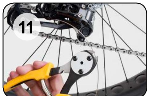
**EN** Cut off excess inner cable.
