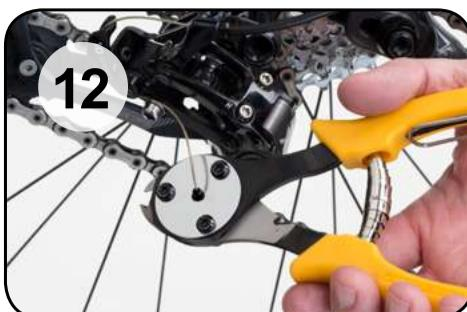
**EN** Install and crimp the cable tip (D).
