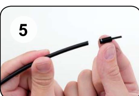
**EN** Use the pre-installed sealed end cap (A) at the shifter.
