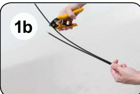
**EN** Alternatively, use the old housing as a reference and cut the new housing to match the length.
