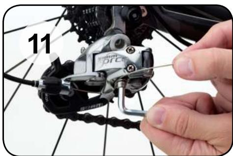
**EN** Tighten anchor bolt and adjust the derailleur per the manufacturer's instructions.
