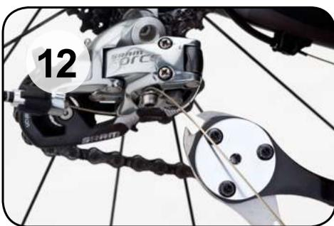
**EN** Cut off excess inner cable.
